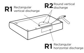
For rectangular ducted discharge installations only. Attach exhaust adaptor/damper over knockout opening with two exhaust adaptor screws. Make sure damper pivot is nearest to top/back edge of
