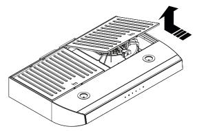
2 Remove the junction box cover. Remove either the top or the back wiring knockout according the preference and install an approved wiring clamp.
