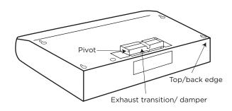
**5** For round ducted discharge installations install 7" (17.8 cm) transition with its screws (2).
