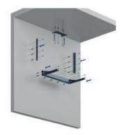
3 Secure the insert hood to the lower support.
