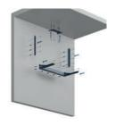
5 Slip the fixed bolts on the shell into the eyelets in the vertical brackets, lay the top of the shell over the ceiling bracket. A solid connection will create a "click".
